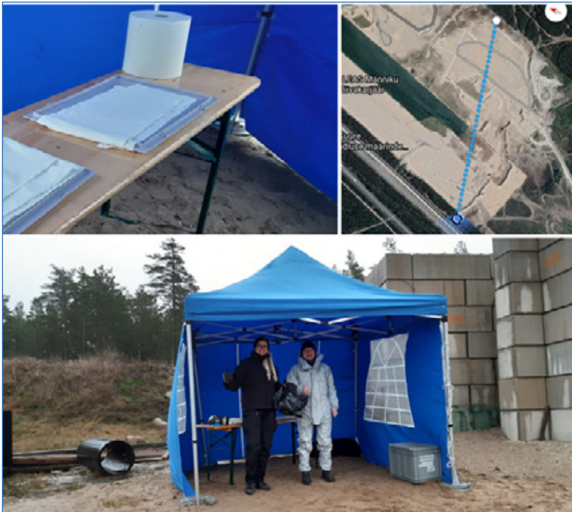
Fig. 3 · Trays for chemical dispersion · Measuring path · Open tent used for the release
