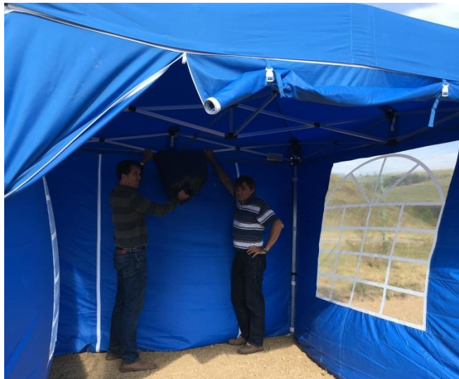
Figure 7 Release of SF 6 into the tent.
